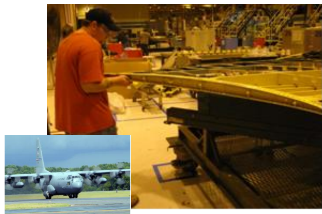
Robins Air Force Base services both cargo and fighter aircraft. The machine shop supports that mission. The technician seen here installs a newly machined part into an aircraft wing section.
