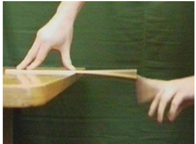
**A way to visualize a natural frequency is to hang a ruler over the edge of a table and flick the end with your finger. The ruler will vibrate at its natural frequency.**
