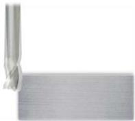
**Force is applied when a tooth of the endmill makes contact with the workpiece. The force causes the endmill to deflect. The amount of the deflection is determined by the depth of cut.**
