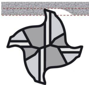
Because the unequal cuts leave a wavy surface, each subsequent pass creates even greater chip thickness variations. This can lead to chatter and it will only get worse. This is what is called "regenerative chatter".
