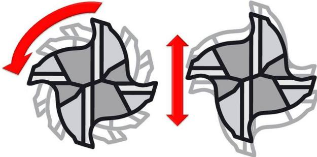
If the back and forth vibration, the tool point's natural frequency, is timed properly with the tooth passing (rotational) frequency, each tooth of the endmill will impact the workpiece at the same instantaneous chip thickness. The cut will be smooth, tool life maximized, the finish superior and the part is accurate.
