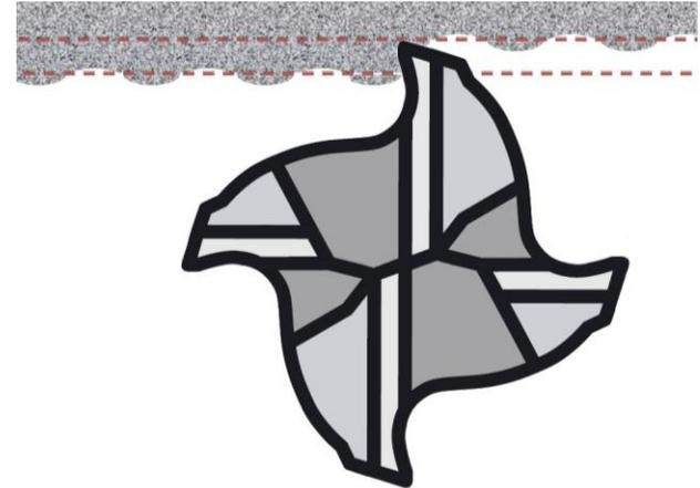
You can overcome the effects of Machining Dynamics by either slowing the spindle speed down enough so that the vibration from one tooth is dissipated before the next tooth comes through or by taking so light a cut that the deflection is miniscule. Machining time will be 5 to 10X longer.
