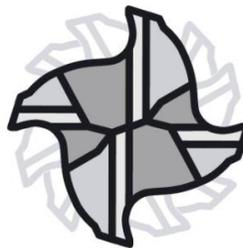
Problem is the vibration is not allowed to fully dissipate. Because the endmill has multiple teeth and is rotating fast, the next tooth impacts the workpiece and the process starts all over again. For example a four flute tool, running at 15,000 RPM, will have 1000 impacts per second.
